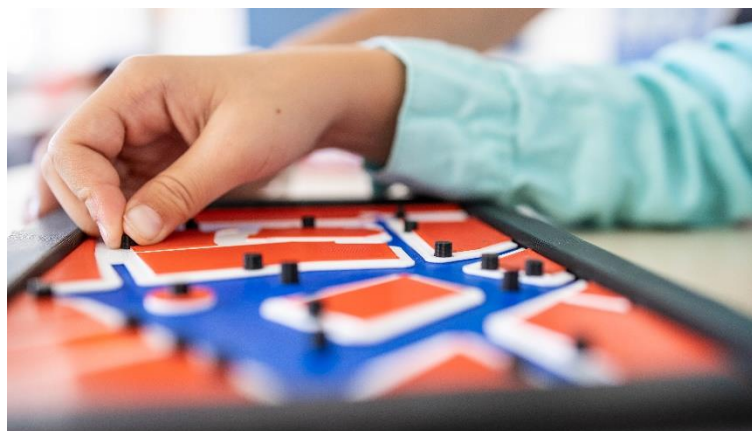
Figure 1. Testing the recognizability of individual shapes of 3D map symbols on a tactile map for people with visual impairment.
