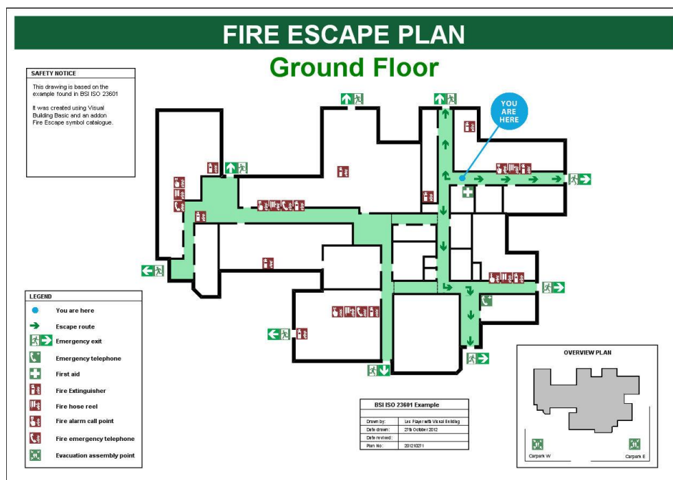
Figure 1. Example of ISO 23601 Escape and Evacuation Plan.
