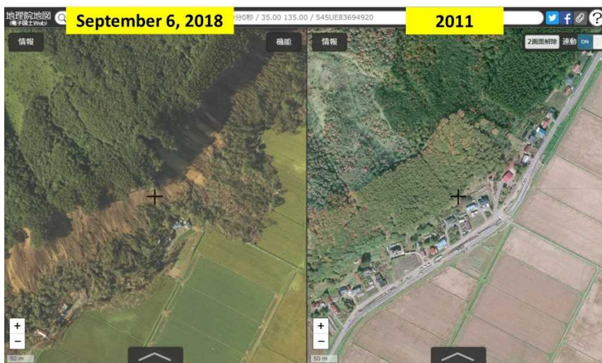
Figure 4. Comparison of aerial photos before and after landslides caused by The 2018 Hokkaido Eastern Iburi Earthquake using two screens display function of GSI Maps
